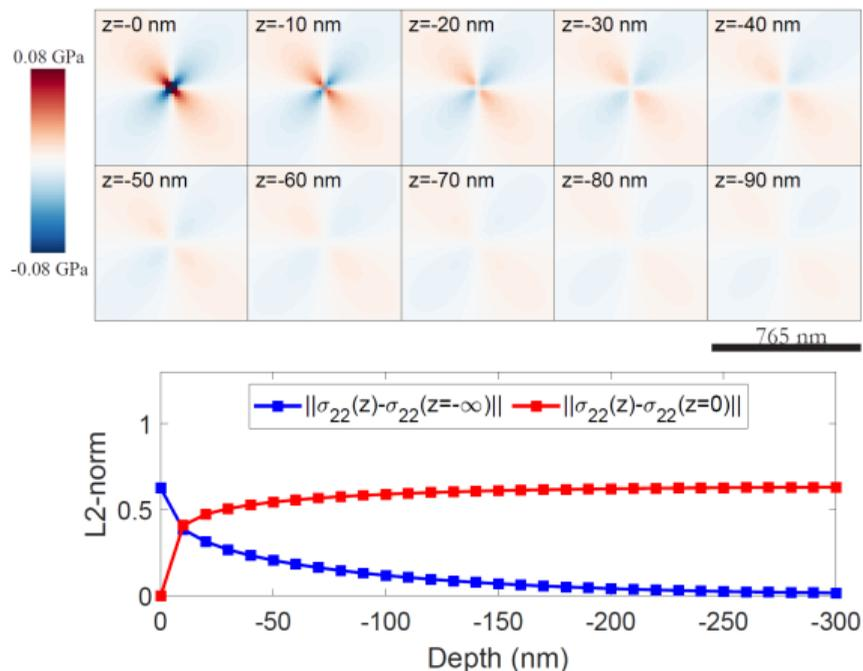
Attenuation of screw dislocation's  $\sigma_{22}$  image stress in the depth ( $-z$ ) direction. Stress maps are plotted from  $z = [0, -90]$  nm.  $L_2$ -norms between  $\sigma_{22}(z)$  and  $\sigma_{22}(z = 0)/\sigma_{22}(z = -\infty)$  are plotted from  $z = [0, -300]$  nm. Stress map color scale range:  $[-0.1, 0.1]$  GPa.
