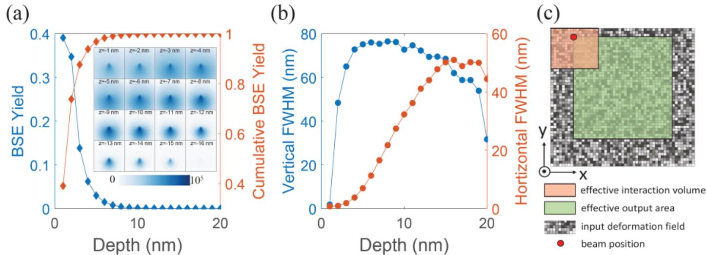
**Figure:** (a) BSE yield and cumulative BSE yield as a function of exit depth, including visualization of the shape of the interaction volume representing the number of electrons from each exit depth bin, (b) vertical/horizontal FWHM of the shape of interaction volume as a function of exit depth, (c) schematic of the effective area (green) probed by an effective interaction volume (red) on a randomly generated grid of deformation field (gray).
