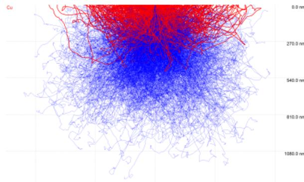
Figure: CASINO MC simulation of Cu at 20kV (Blue:BSE, Red:SE)
