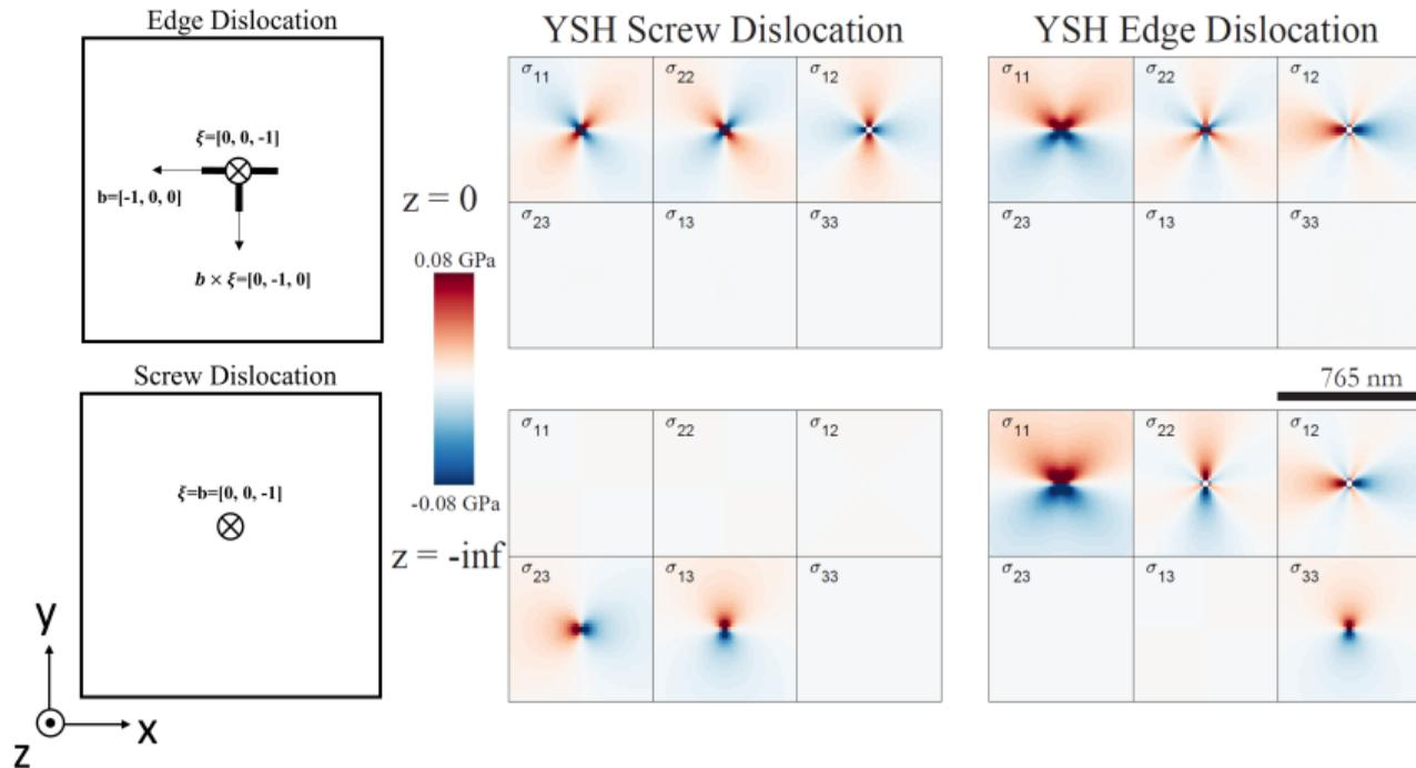
**Figure:** Stress tensor components derived from the YSH model for pure screw and edge dislocations at  $z = 0$  and  $z = -\infty$ . Each box represents a map of a particular tensor component with a box dimension of  $765 \times 765 \text{ nm}^2$  and 3 nm pixel size.
