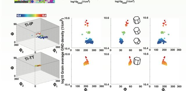
➢ The order of magnitude of grain average GND density is linearly dependent on the  $\Phi$  angle.
