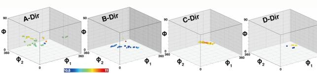
➢ Orientation dependence of the grain average GND density is negligible.
