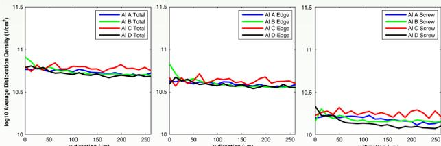
➢ Higher GND density close to center of shear band for B-Dir and across the C-Dir lead to pronounced strain hardening effect. Hence, they retain higher peak loads.
