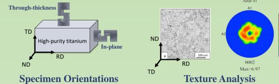
**Materials:** High-purity titanium with strong in-plane basal texture (Gray *et al.*, 2016). The in-plane specimen's shear plane is aligned to the basal texture whereas the through-thickness specimen retains a non-basal texture. They are both quasi-statically compressed at a strain rate of 0.001/sec at 298K.
