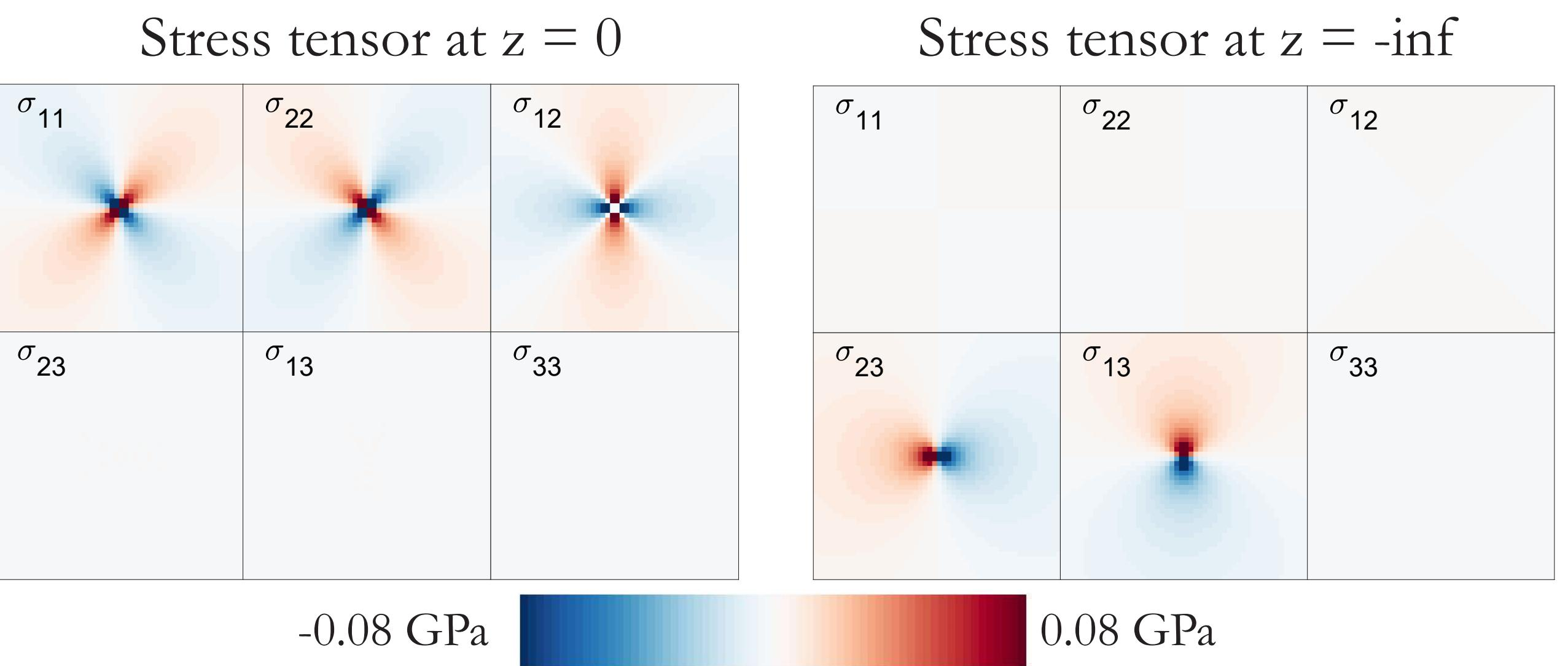
Image stress attenuation for  $\sigma_{22}$  along the depth direction
